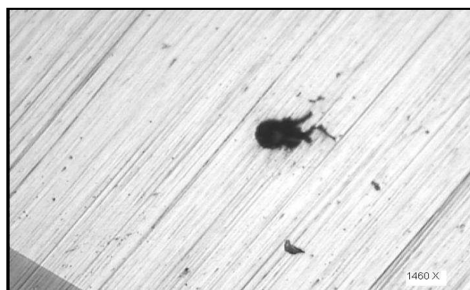
Figure 6 – Pitting visible on the surface of retractor A after polarization assay using enzymatic detergent solution (730 x magnification).
